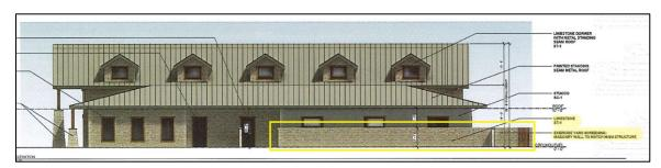
Figure 2. Exhibit "C" of Ord 454 shows elevation of exercise yard fence, boxed in yellow.
